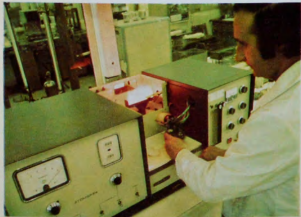
Left. Quality control at Rover not only takes in the machined and finished components but also the basic materials from which they are made. An Atomic Absorption Spectrometer is used in the final element analysis of 'bought-in' metals to establish whether they comply with the exacting specifications required.
