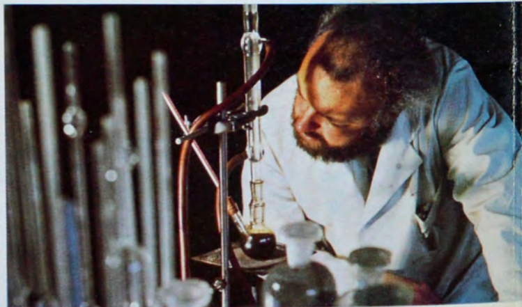
Left. Every day, samples of hydraulic brake fluid are taken from the assembly lines where braking systems are filled, and their boiling point is checked. A low boiling point indicates the presence of atmospheric moisture in the fluid. Where safety is concerned, no risks are taken.
