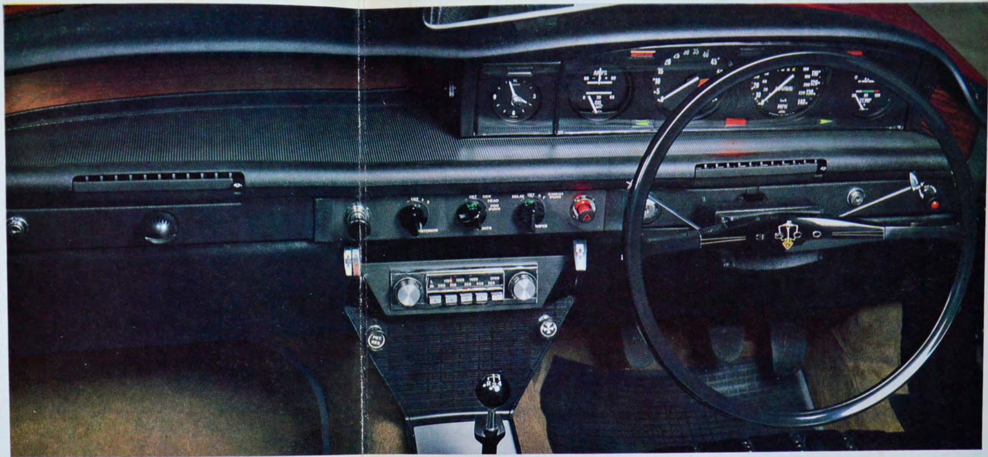
Above. The instrument display is directly in the driver's line of sight and clearly visible through the top half of the steering wheel when suitably adjusted. Two finger-tip control stalks below the steering wheel operate headlamp dip/flash systems, and direction indicator and horn respectively. All other controls and switches are within easy reach.
