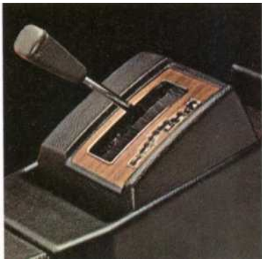
An optional 3-speed automatic transmission with illuminated, floor-mounted gear selector is available.
