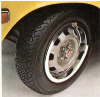
Low profile radial ply tires are standard equipment on all live wheels.
