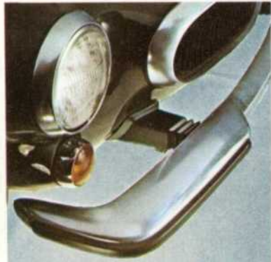
But new bumpers aren't designed to bump but rather, to take a bumping. They're mounted on oil-filled, hydraulic shock absorbers and designed to take impacts at 5 mph (front) and 2.5 mph (rear).
